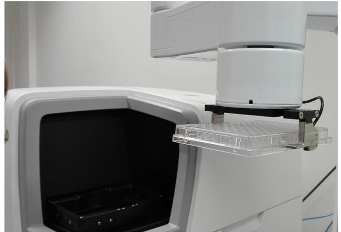
**Figure 2** Installation of KX-2 robot, Celldiscoverer 7 and incubator at a customer site
